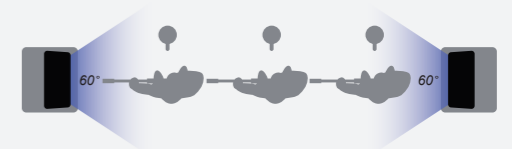
Side Fills: P12 wedges (standard horn) on L15 subs on each side
